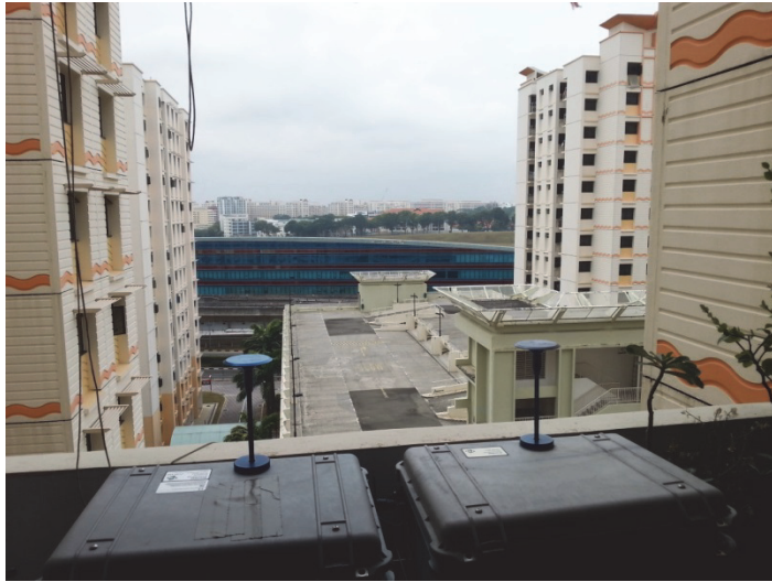
Figure 1. Co-located DustTrak Monitors inside Environmental Enclosures (Model 8535) in Singapore
