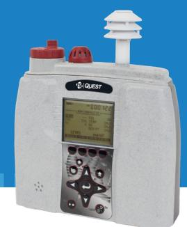
The TSI® Quest™ EVM Environmental Monitors simultaneously measure particulates and gas concentration in real-time. These monitors measure select toxic gases, volatile organic compounds (VOCs), relative humidity and temperature.
