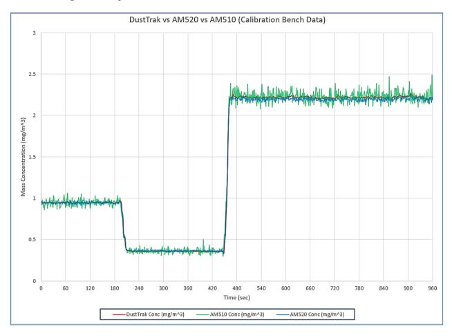
As the graph above shows, each instrument will have a unique response signature to the same aerosol, with the SidePak AM510 showing the most variability. However, the correlation of all three instruments are very similar with the DustTrak II monitor and SidePak AM520 being very closely aligned.
