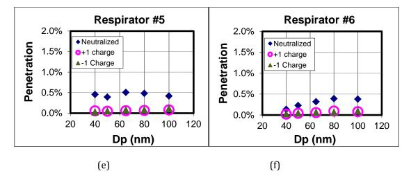
Figure 2: Percent Penetration vs. Particle Size Curves for Various N95 Filtering-Facepiece Respirators
