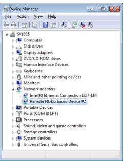
The driver function can be confirmed by looking into the computer's device manager. The instrument will show up as a Remote NDIS device under Network Adapters (see screen capture below).
