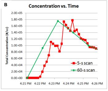
Figure 3: (A) Mean size and (B) total concentration vs. time during toaster operation, measured with 5-s scans and 60-s scans.
