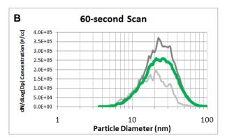
Figure 2: Particle size distributions during toaster operation, measured with (A) 5-s scans and (B) with 60-s scans.
