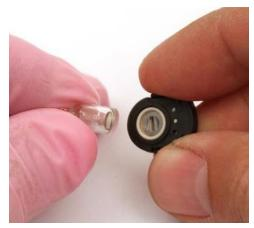
Figure 37: Reinstalling the Electrode Lamp
