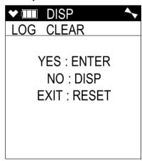
To continue through Display Mode without clearing the log data, press and release the **DISP/LOCK** button.
