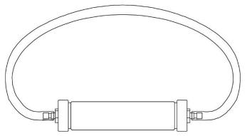
Figure 53: Reconnect Tubing to Dehumidifier Filter
