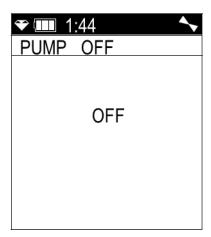
2. To turn the pump back on and continue in Display Mode or return to Measuring Mode, press and release the **DISP/LOCK** button.
