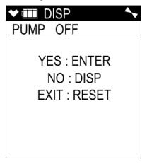
In this screen, press and release the **POWER/ENTER** button to turn the pump off. The fan symbol in the upper right corner will disappear. Once the pump is off, you cannot exit this screen and return to Measuring Mode or continue in Display Mode until you turn the pump back on.
