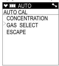
4. If you were using a 5-gas (standard 4-gas plus ESS-03) calibration cylinder to calibrate the standard 4 sensors, continue to Step 5.
