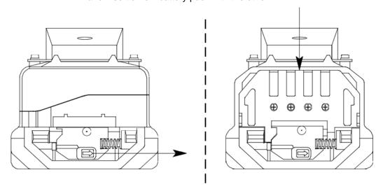
Be sure Battery Pack Release Latch is Pushed to the Right
