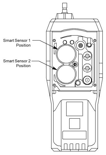
Figure 44: Smart Sensor Positions
