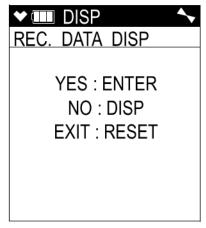
1. With the snap logging screen displayed, press and release the **POWER/ ENTER** button. The screen that appears will depend on whether or not any snap logs have been taken.
