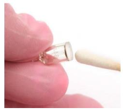
Figure 30: Polishing the Electrode Lamp Window
