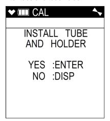
4. Be sure a filter tube is installed in the tube holder and then attach the tube holder to the instrument's inlet fitting. See "Replacing a Tube" in Appendix I for instructions.
