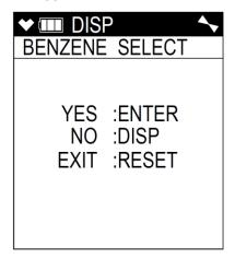
• The PID Gas Name Screen operates as described in "<u>PID Gas Name Screen</u>" in Chapter 3 but is factory set up for and calibrated to benzene and appears as shown below. If there are 2 PID sensors installed in your GM460, the PID Gas Name Screens will appear in Display Mode in the following order regardless of their position in the flow system: 10.0 eV/benzene, 10.6 eV, 11.7 eV.
