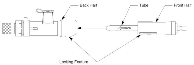
Figure 49: Reassembling Tube Holder
