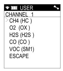
5. Use ▲ AIR and SHIFT ▼ (PANIC) to move the cursor next to the desired configuration for the selected channel. In the example below, the cursor has been moved next to the H2S (H2S) selection.
