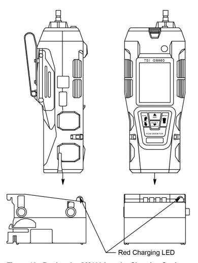
Figure 18: Putting the GM460 into the Charging Station
