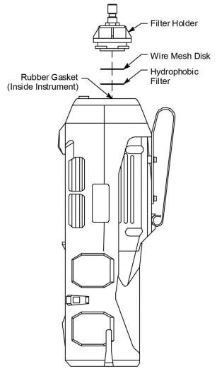
Figure 27: Changing the Filter and Wire Mesh Disk
