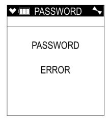
You must turn the unit off and reenter Maintenance Mode 2 using the correct password.
