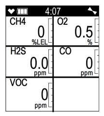
7. To change operating modes by returning to the Mode Select Screen, press and hold the ▲ AIR and DISP / LOCK buttons for 5 seconds.
