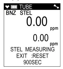
c. To cancel the STEL measurement, press and release the RESET button. Then press and release the POWER/ENTER button.
