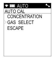
7. Press and release the POWER/ENTER button. The first of the Gas Select Screens, the standard four sensors screen, will be displayed. In addition to the standard four sensors screen, there is a separate screen for each installed smart sensor, and an ESCAPE screen that will take you back to the Auto Cal menu. Use the ▲AIR and SHIFT ▼(PANIC) buttons to scroll through the different screens.
