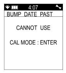
The GM460 cannot be used until a successful bump test has been performed. Press and release the **POWER/ENTER** button to enter Calibration Mode. See <a href="Chapter 4">Chapter 4</a>, "Calibration Mode" for instructions to bump test the GM460.
