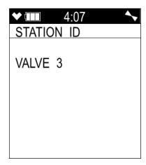
3. Use the ▲AIR and SHIFT ▼(PANIC) buttons to scroll to the desired Station ID then press and release the POWER/ENTER button to return to the Snap Logging Screen sequence.
