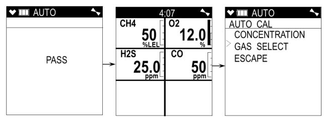
20. If any of the sensors cannot be adjusted to the proper value, a screen displays that indicates a calibration failure and lists the sensor(s) that failed to calibrate. In the example below, the oxygen and  $H_2S$  channels failed calibration. The other sensors calibrated normally.
