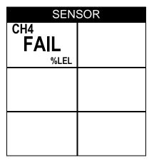
To continue, press and release the **RESET** button to acknowledge the failure. The gas reading for the failed sensor will be replaced by "- - - -". Replace the failed sensor as soon as possible.
