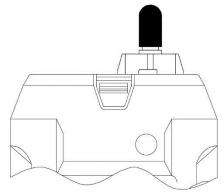
Figure 52: Plug Inlet Fitting with Black Rubber Cap
