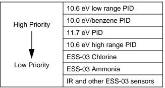
For example, if your instrument is a 4-gas + high range PID + IR HC, the high range PID sensor should be in the smart sensor 1 position and the IR HC sensor should be in the smart sensor 2 position. If your instrument is a 4-gas + IR HC, the IR HC sensor should be in the smart sensor 1 position and a dummy sensor should be installed in the smart sensor 2 position. See the figure below for the location of the smart sensor 1 and 2 positions.
