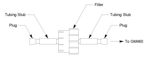
Figure 41: VOC Zero Filter
