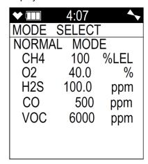
Use the ▲AIR or SHIFT ▼(PANIC) button to scroll to the Bar Hole Mode Select Screen.
