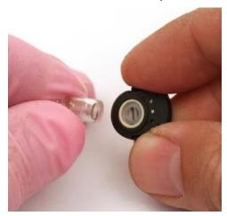
Figure 34: Reinstalling the Electrode Lamp
