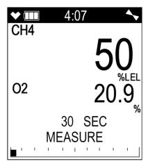
6. At the end of the sample period, the pump will shut off and the buzzer will sound then the peak combustible gas reading and the minimum oxygen reading for the sample period will be displayed. The peak combustible gas reading will also be visually displayed on the graph along the bottom of the screen.
