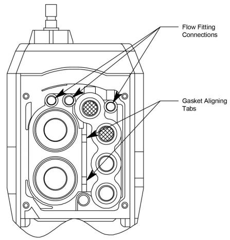
Figure 35: Sensor Gasket Seating
