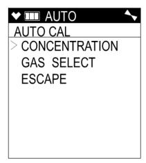
6. To check or update the gas concentrations, use the ▲AIR and SHIFT ▼ (PANIC) buttons to put the cursor next to CONCENTRATION and press and release the POWER/ENTER button to display the Calibration Gas Values Screen.
