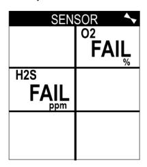
The buzzer and alarm LEDs activate in a double pulsing pattern. Press and release the **RESET** button to reset the alarm and continue to the Auto Cal Menu. After calibrating the PID channel by following the instructions below, attempt to calibrate the standard channels again. If the failure continues, investigate the cause. See "Troubleshooting" in Chapter 6.
