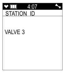
3. Use the ▲AIR and SHIFT ▼(PANIC) buttons to scroll to the desired station ID and press and release POWER/ENTER. The unit will return to the Bar Hole Measuring Screen.
