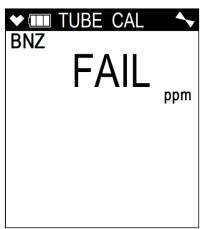
Press and release the **RESET** button to clear the alarm and return to the **TUBE CAL** Auto Calibration Menu. See "<u>Troubleshooting</u>" in Chapter 6.
