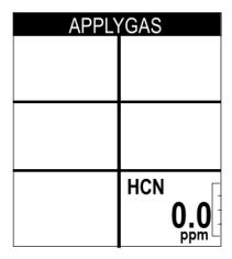
If you do not want to proceed with the calibration, press and release the **DISP/LOCK** button to return to the Gas Select Screen.
