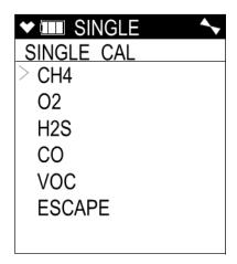
Move the cursor next to the sensor you want to calibrate with the ▲AIR and SHIFT ▼ (PANIC) buttons. In the example above, the CH4 sensor is selected for span adjustment.
