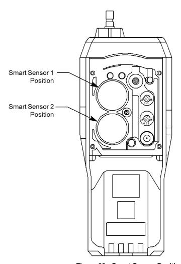
Figure 39: Smart Sensor Positions
