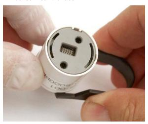
Figure 28: Using Removal Tool
