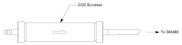
Figure 42: CO<sub>2</sub> Scrubber Connected to GM460
