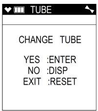
Once the tube is changed, press and release the POWER/ ENTER button to start the measurement. Return to Step 8.
