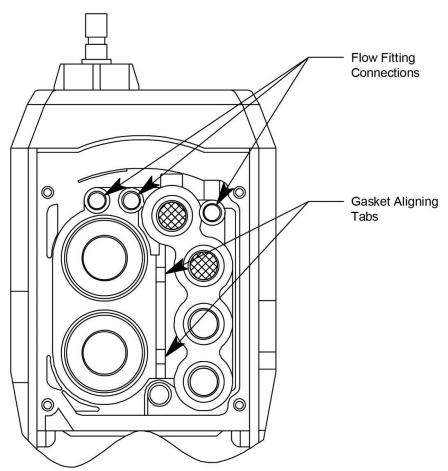
Figure 26: Sensor Gasket Seating
