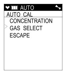
15. Press and release the **POWER/ENTER** button. The first of the Gas Select Screens, the standard four sensors screen, will be displayed. In addition to the standard four sensors screen, there is a separate screen for each installed smart sensor, and an **ESCAPE** screen that will take you back to the Auto Cal menu. Use the ▲ AIR and SHIFT ▼ (PANIC) buttons to scroll through the different screens.
