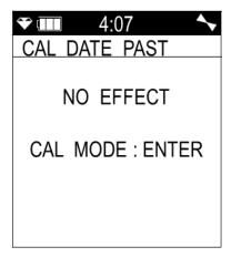
To enter Calibration Mode, press and release the **POWER/ENTER** button. If you do not want to enter Calibration Mode, wait for the instrument to continue with its startup sequence.
