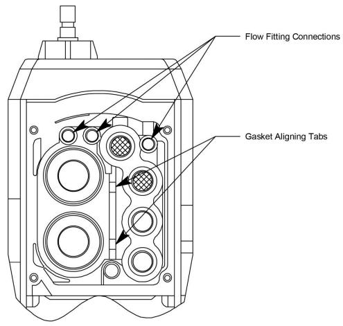
Figure 24: Sensor Gasket Seating
