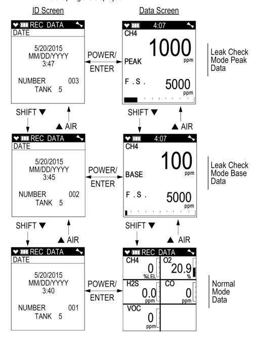
Snap log data that was taken in Leak Check Mode operation will have 2 sequential screens that are part of one data set. One screen is for the base reading and the other screen is for the peak reading. "BASE" and "PEAK" will appear in the gas reading screen for each type of reading, respectively. If a base data point appears without a peak data point after it, it is because a peak data point was not taken.
