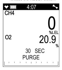
• When the purge is complete, the screen will return to the initial Bar Hole Mode screen.
