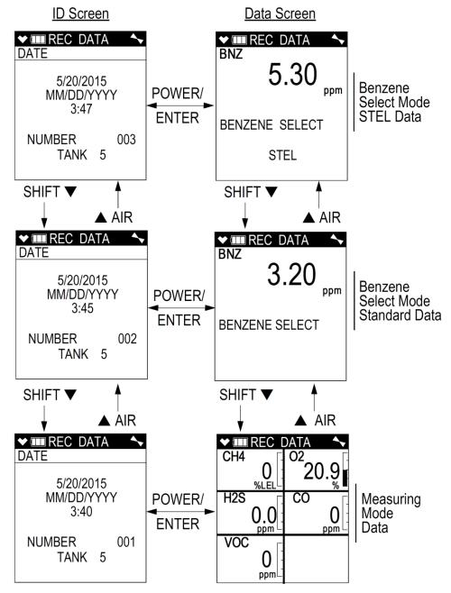
The instrument saves data from a Benzene Select Mode standard measurement and from a Benzene Select Mode **STEL** measurement (if performed). Data from a Benzene Select Mode standard measurement will say "**BENZENE SELECT**" below the reading. Data from a Benzene Select Mode STEL measurement will say "**BENZENE SELECT**" and "**STEL**" below the reading. They are separate files. Data may also be present from snap log data saved in Measuring Mode.
