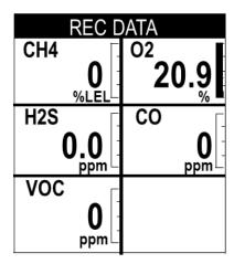
The gas readings that were taken during the snap log are displayed. You can use the ▲AIR and SHIFT ▼(PANIC) buttons to scroll through the different snap logs. The gas readings will change as you view different snap log data but the snap log ID is not visible from this screen. To scroll through the data by viewing the snap log ID number, press and release POWER / ENTER.
