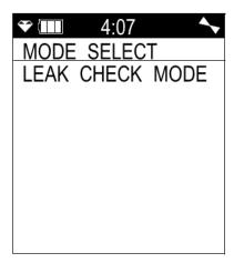
With the Leak Check Mode Select Screen displayed, press and release the **POWER/ENTER** button to begin the Leak Check Mode startup sequence.
