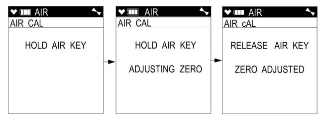
9. Release the ▲ AIR button. The fresh air adjustment will finish, the fresh air readings will be displayed momentarily, and then the instrument will return to the Calibration Mode Screen.
