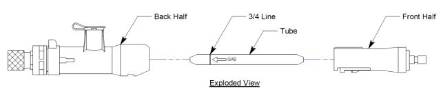
Figure 46: Tube Holder Component Location
