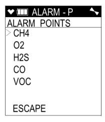
3. Move the cursor next to the channel of the alarm point you want to update. Press and release **POWER/ENTER**. The channel's alarm points and alarm operation (oxygen only) are displayed.
