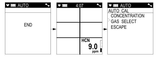
If the ESS-03 channel cannot be adjusted to the proper value, a screen displays that indicates a calibration failure and indicates that the ESS-03 sensor failed to calibrate.
