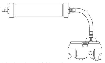
Figure 51: Connect Tubing to Inlet
