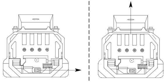
Slide Battery Pack Release Latch to the Right
