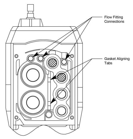
Figure 38: Sensor Gasket Seating
