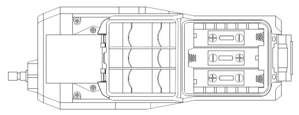
Figure 13: Installing the Alkaline Batteries
