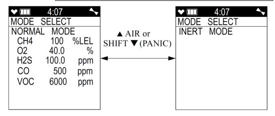
4. With the Inert Mode Select Screen displayed, press and release the **POWER/ENTER** button to begin the Inert Mode startup sequence.
