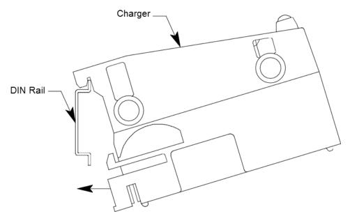
Figure 6: Installing a Charger on the DIN Rail
