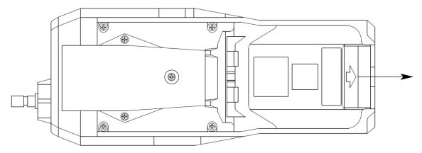
Figure 11: Releasing Battery Cover Latch
