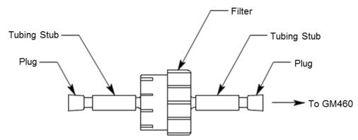
Figure 3: VOC Zero Filter
