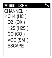
6. Press and release **POWER/ENTER** to select the channel configuration.
