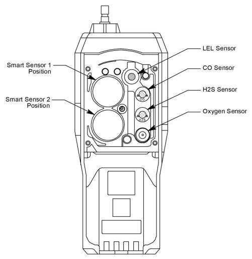
Figure 25: Replacing a Sensor
