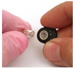
Figure 31: Reinstalling the Electrode Lamp
