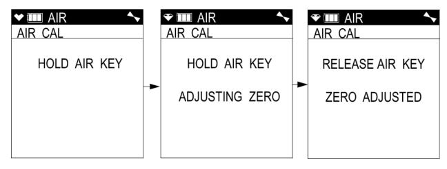
6. Release the ▲ AIR button. The fresh air adjustment will finish, the fresh air readings will be displayed momentarily, and then the instrument will return to the Calibration Mode Screen.
