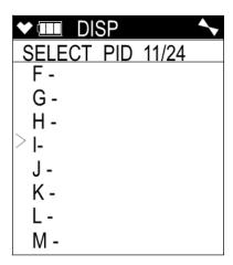
2. Use the ▲AIR and SHIFT ▼(PANIC) buttons to scroll through the letter and list options. To view the gas names behind a letter, User List, or Recent List, press and release the POWER/ENTER button when the cursor is next to the desired letter.
