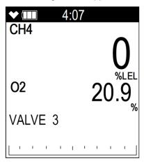
7. The combustible gas and oxygen channels are displayed along with the battery charge level and station ID.
