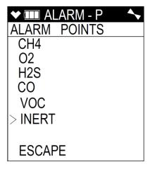
2. Select **INERT** (not **O2**) in order to view or change Inert Mode's oxygen alarm points.
