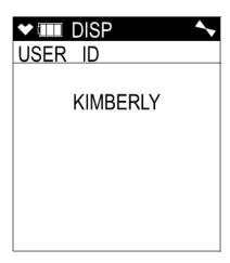
The user ID provides a way to identify the GM460 user during a data logging session. If the user ID is changed during an operating session, a new data session is initiated with the new user ID attached to it. This allows you to change the user ID during operation and have each user ID that was used during an operating session saved for the corresponding data. See the GM460 Data Logger Management Program Operator's Manual (P/N 6011446) for a detailed description of data logging and the user ID.
