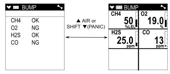
b. To return to the Gas Select Screen, press and release the POWER/ ENTER button. If any channel failed the bump test, the buzzer will sound a double pulsing tone until you press and release the POWER/ ENTER button.
