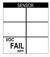
The buzzer and alarm LEDs activate in a double pulsing pattern. Press and release the **RESET** button to reset the alarm and continue to the Auto Cal Menu. Attempt to calibrate the PID channel again. If the failure continues, investigate the cause. See "<u>Troubleshooting</u>" in Chapter 6.
