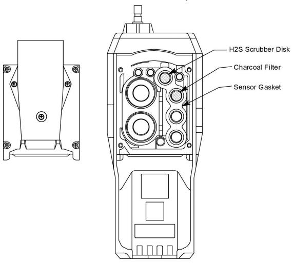
Figure 23: Replacing the H<sub>2</sub>S Scrubber Disk and Charcoal Filter
