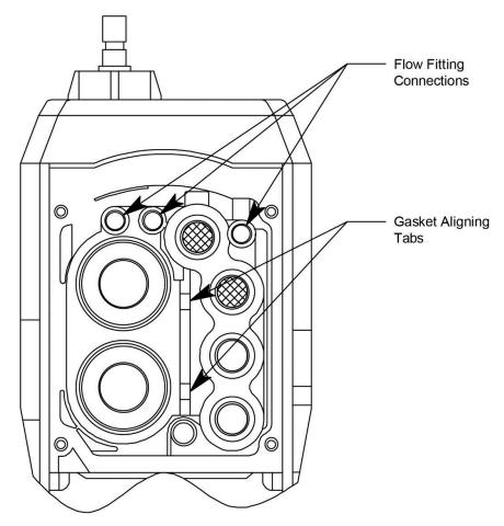
Figure 32: Sensor Gasket Seating
