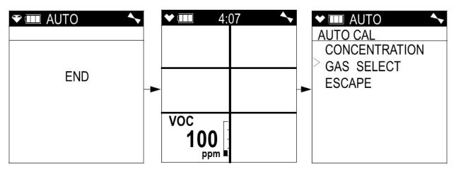
If the PID channel cannot be adjusted to the proper value, a screen displays that indicates a calibration failure and indicates that the PID sensor failed to calibrate.
