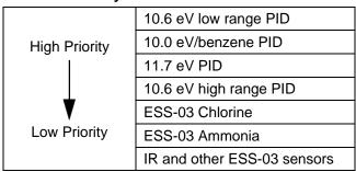
For example, if your instrument is a 4-gas + low range PID + high range PID, the low range PID sensor should be in the smart sensor 1 position and the high range PID sensor should be in the smart sensor 2 position. If your instrument is a 4-gas + high range PID, the high range PID sensor should be in the smart sensor 1 position and a dummy sensor should be installed in the smart sensor 2 position. See the figure below for the location of the smart sensor 1 and 2 positions.
