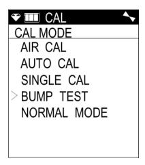
8. Press and release the POWER/ENTER button. The first of the Gas Select Screens, the standard four sensors screen, will be displayed. In addition to the standard four sensors screen, there is a separate screen for each installed smart sensor, and an ESCAPE screen that will take you back to the Calibration Mode menu. Use the ▲AIR and SHIFT ▼(PANIC) buttons to display the gas(es) you want to test.
