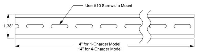
Figure 5: DIN Rail Dimensions
