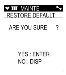
5. Press and release the **POWER/ENTER** button. The screen will indicate that the default configuration has been restored and return to the main menu.
