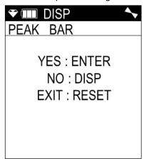
With the Peak Bar Screen displayed, press and release the POWER/ ENTER button. The current setting will be displayed.
