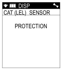
With the CAT (LEL) SENSOR PROTECTION screen displayed, press and release the POWER/ENTER button. The current setting will be displayed along with a warning about no %LEL alarms if the catalytic LEL sensor is turned off.
