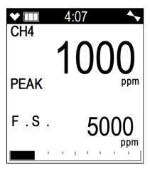
10. Take the instrument to the monitoring area. The instrument will retain and display the highest gas concentration encountered.
