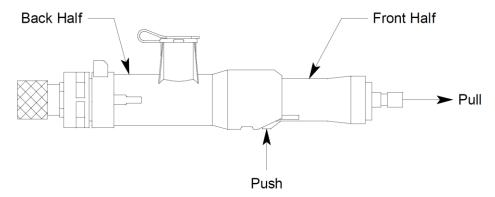
Figure 47: Replacing a Tube
