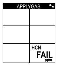
The buzzer and alarm LEDs activate in a double pulsing pattern. Press and release the **RESET** button to reset the alarm and continue to the Auto Cal Menu. Attempt to calibrate the ESS-03 channel again. If the failure continues, investigate the cause. See "Troubleshooting" in Chapter 6.
