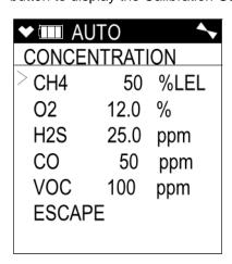
The gas concentrations displayed in the Calibration Gas Values Screen must match the gas concentrations listed on the 5-gas cylinder or the 4- gas calibration cylinder and the PID cylinder.
