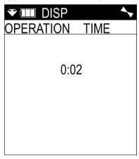
If **LUNCH BREAK** is set to **ON**, the time in operation will only be reset if you do not choose to resume the peak and TWA measurements when the GM460 is turned on in the Lunch Break Screen described in Step 3 in "Turning On the GM460" in Chapter 3. If you choose to resume the peak and TWA measurements during startup, the GM460 will include the time in operation when the unit was last turned off in the current time in operation.
