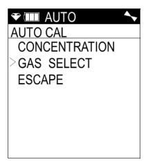
24. Press and release the **POWER/ENTER** button. The first of the Gas Select Screens, the standard four sensors screen, will be displayed. In addition to the standard four sensors screen, there is a separate screen for each installed smart sensor, and an **ESCAPE** screen that will take you back to the Auto Cal menu. Use the ▲ AIR and SHIFT ▼(PANIC) buttons to scroll through the different screens.
