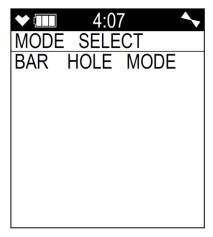
4. With the Bar Hole Mode Select Screen displayed, press and release the **POWER/ENTER** button to begin the Bar Hole Mode startup sequence.
