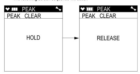
2. Release the **RESET** button. The peak readings will be reset and the unit will return to the Peak Screen.
