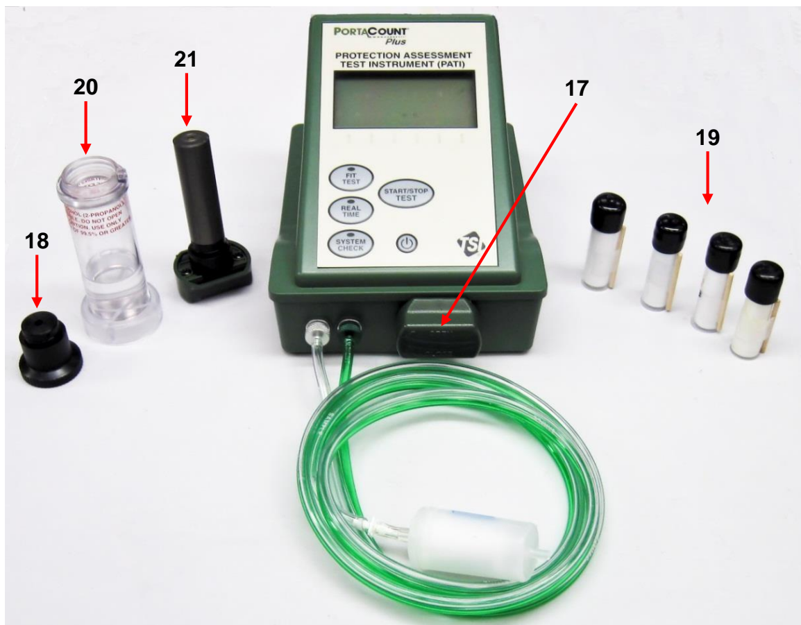
Operational Components and Cartridge Cavity
