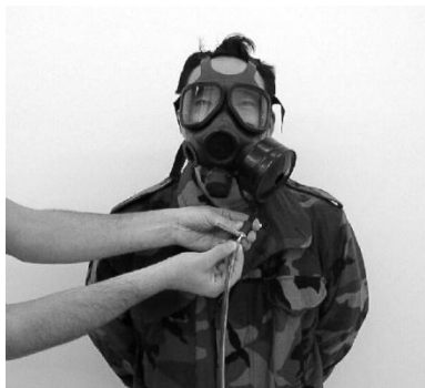
Connecting PATI Sample Line to Drink Tube Sampling Adapter
