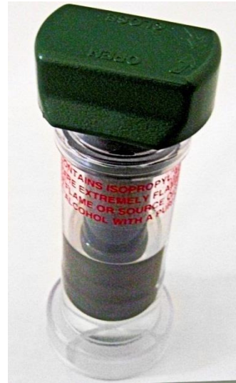
Alcohol Cartridge Properly Stored in Alcohol Fill Capsule
