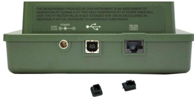
Plugs for the USB Connector and the Data Port
