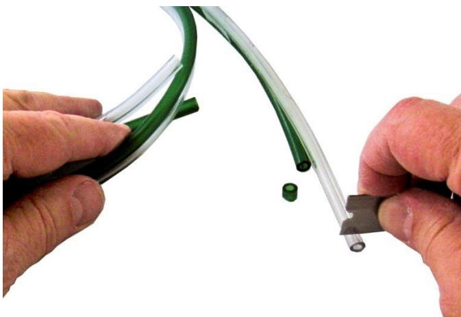
Trimming the Twin Tube Assembly
