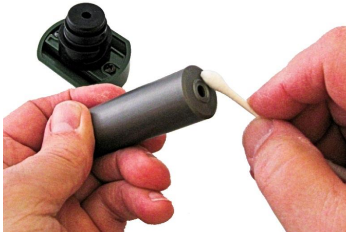
Cleaning the Alcohol Cartridge and Storage Cap
