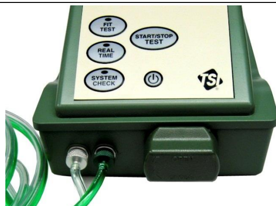
Alcohol Cartridge Correctly (Fully) Seated
