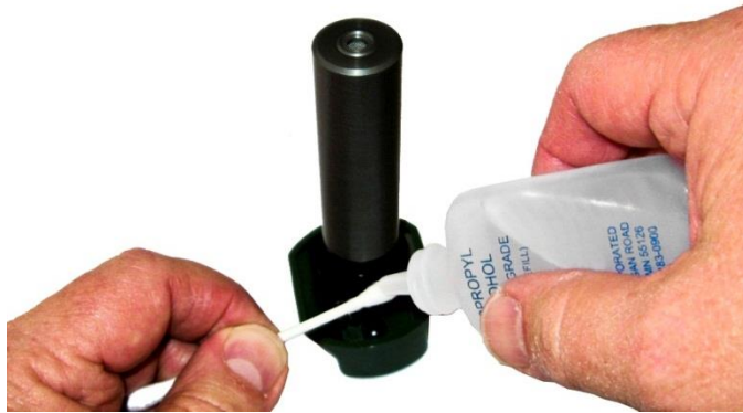
Applying Alcohol to Applicator
