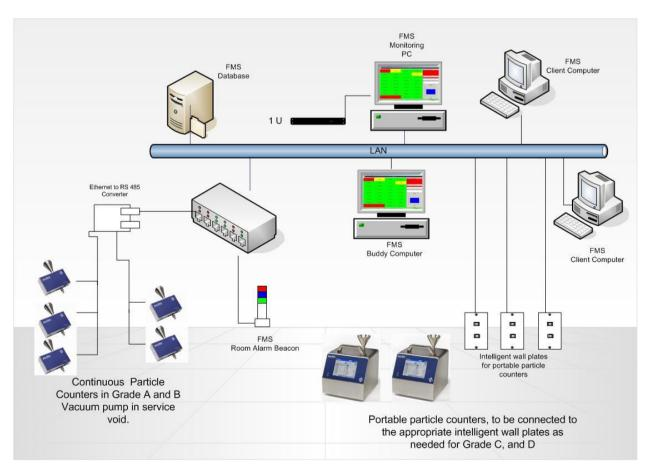
Figure 1 Typical FMS System Utilizing Traditional Particle Counters
