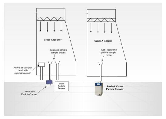
Figure 6. Three Measurements with a Single Sample Probe
