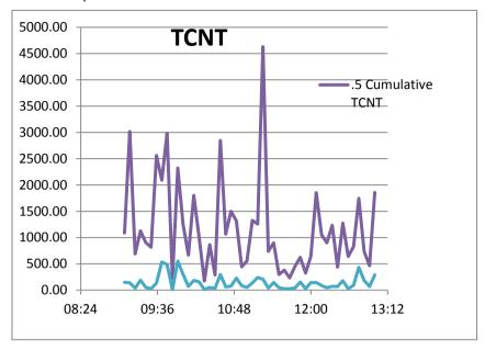
Figure 2.TCNT - Total Particle Counts at ≥0.5 µm and ≥5 µm
