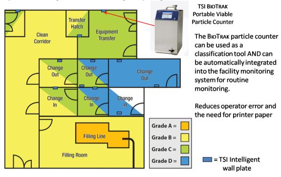
Figure 7. Example of a Cleanroom with Wall-Plate Access for use with BioTrak Particle Counter in Grade C and D Environments
