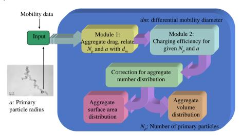
Figure 1. Two module approach for nanoparticle aggregate mobility analysis. Courtesy: Lall, et al., 2006 c
