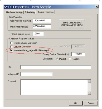
Figure 2. Physical properties tab of the Aerosol Instrument Manager® software showing the nanoparticle aggregate mobility analysis module user interface.
