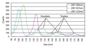
Typical resolution is within 2.5% of the particle diameter at 0.1  $\mu$ m. The Laser Aerosol Spectrometer can differentiate between 100 nm and 107 nm PSL!
