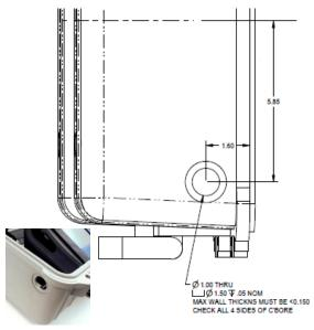
2. The Environmental Enclosure Bracket may need two holes added. Check the back left section of the large black sheet metal bracket for the installed 6-32 PEM nuts.
