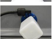
Install the Heated Inlet on top of the Auto-Zero 3. Module.
