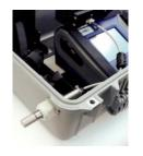
Attach Power Cable for Model 8535 to incoming power, DustTrak<sup>™</sup> monitor, and Heated Inlet.
