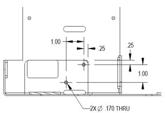
5. Then use two 6-32 locking nuts on the back side of the flange when attaching the "Mounting Bracket."
