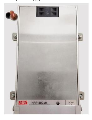
3. Using a 7/16" socket on a socket wrench, install the 4 nuts and washers (hand tight) to secure to the power supply to the threaded studs.
