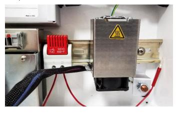
9. Insert the #2 wire from the right side of the Thermostat into the left side of the heater connector.
