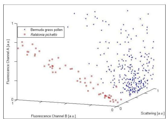
Figure 4B. Raw Data with Three Discrimination Parameters: Particle Size, Fluorescence A, and Fluorescence B
