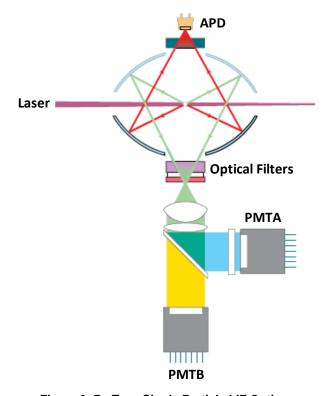
Figure 3. BIOTRAK Single Particle LIF Optics
