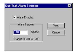
4. Turn "On" the alarm function by checking the "Alarm Enabled" check box. Enter a value within the acceptable range. In this example, the DustTrak™ monitor is programmed to a setting of "0.100 mg/m³." Press the **Send** button, to program the instrument.
