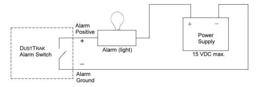
Since applications of this function will vary, TSI supplies only the output cable (part no. 801652). The output cable is labeled with the pin-out wiring diagram. The user is responsible for all additional equipment needed for making connections to their own equipment.
