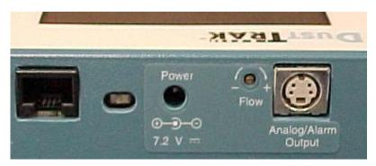
**Note:** For technical information on using the DUSTTRAK™ monitor's analog output features see Application Note ITI-073, Analog Output on the TSI Website at www.tsi.com.
