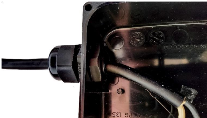
Figure 7: Strain Relief and Power Cable through Access Hole
