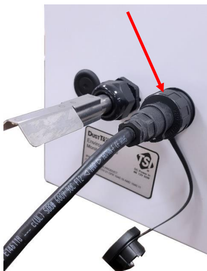
Figure 23: Power Cord from Solar Battery to Environmental Enclosure
