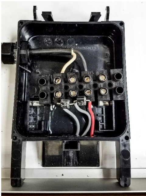
Figure 10: Attach Power Cable to Screw Terminals
