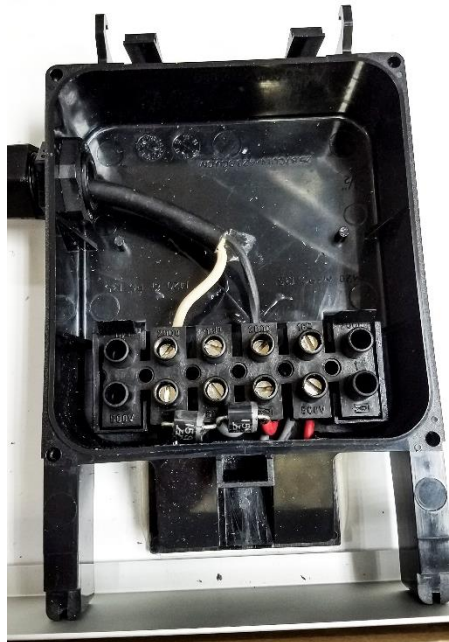
Figure 11: Secure Terminal Block and Tighten Strain Relief
