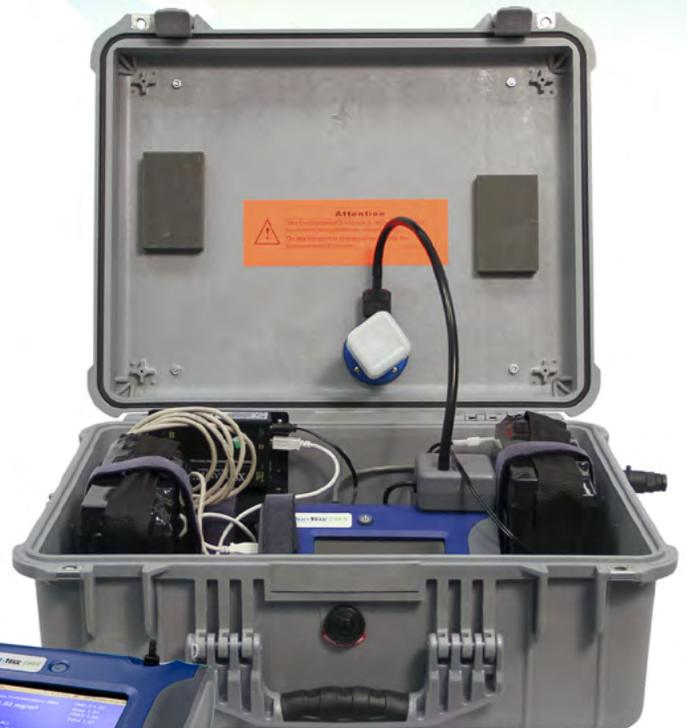
2-in-1 - Remove DustTrak II from the case for use as a smaller desktop monitor, indoors or out.
