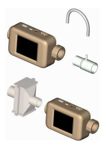
5. Insert alternative Tube Ends into the inlet of the Filter and into the outlet side of the Airway Pressure Fitting.
