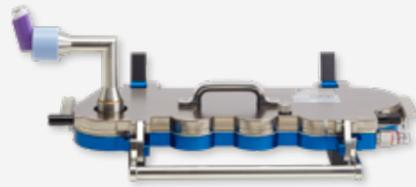
The recommended test set-up is with an NGI, but an ACI may also be used. Impactors with 7 or 8 stages are preferred by regulators, as they provide good APSD resolution. However, for some established methods the MSLI or GTI may be acceptable.
