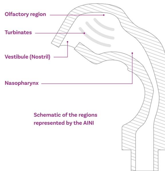
Understanding and optimising regional deposition is essential to maximise the fraction of drug absorbed via the target pathway and to minimise drug transit to the lungs. For nasally inhaled products, the AINI enables representative testing of the deposition of drug within the nasal airways
