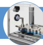
The NGI Cooler can only be used for nebulisers with mouthpieces. For nebulisers with facemasks the NGI will need to be removed from the NGI Cooler for testing, once the required temperature has been reached.
