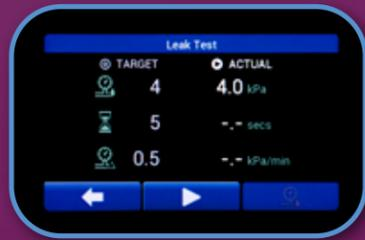
Leak test screen
