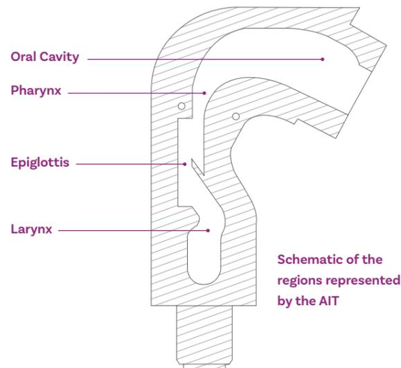
For orally inhaled products (OIPs), the AIT provides analysts with data more representative of measured *in vivo* behaviour, by ensuring that the ISM corresponds with the portion of the aerosol that would likely enter the lungs.
