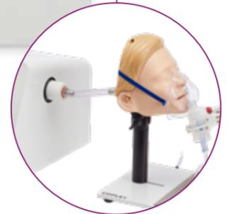
Inlet/outlet port for direct connection to the dose filter holder and nebuliser, spacer or VHC
