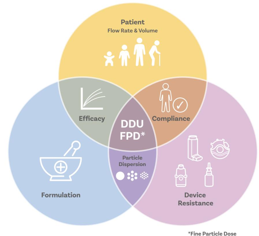
In this environment, accuracy and sensitivity alone do not maximise the utility of *in vitro* testing. Due to the complex interactions between formulation and device and the impact of patient-to-patient variability, identifying robust relationships between product characteristics and clinical efficacy can be challenging - very few good IVIVCs exist for OINDPs.
