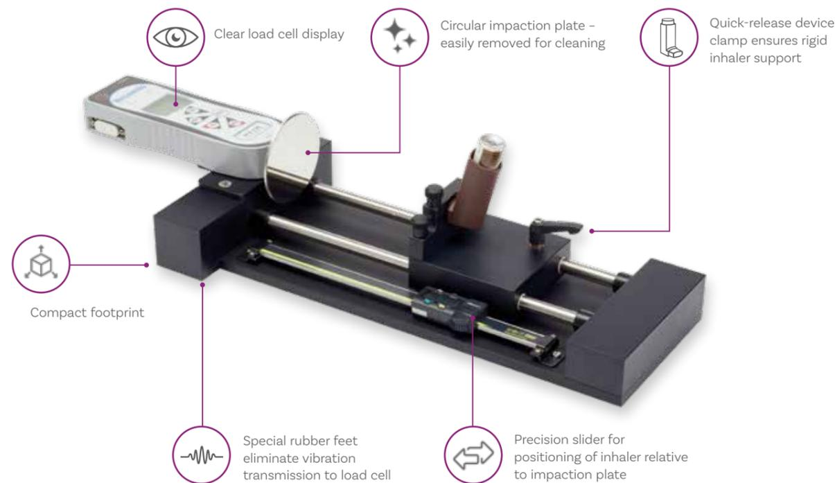
A sample of the inhaler to be tested is required at the time of placing an order so that a customised clamp can be made.
