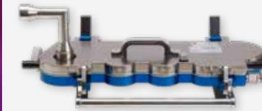
The test set-up is shown with an NGI but an ACI is equally suitable for the assessment of nasal powders. The Fast Screening Andersen (FSA) impactor is a reduced stack plus filter version of the ACI. As little deposition is expected in the lower stages, the FSA may be used to assess the APSD characteristics of nasal powders.
