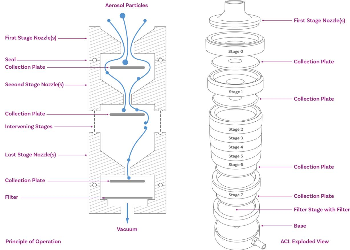
Unlike the NGI, the stages of the ACI are arranged vertically. The aerosol flow passes first through the stage at the top of the impactor, through to the last stage and a final filter at the bottom of the impactor arrangement.
