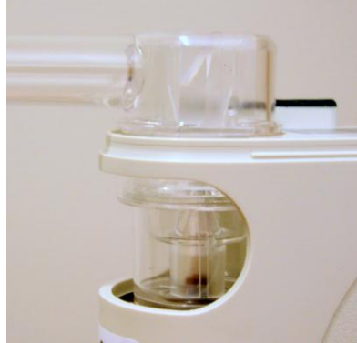
Figure 4. Plug Cartridge and Elbow into the Top of Qfit™ Tester
