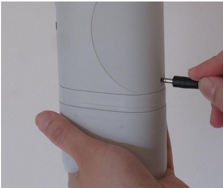
Figure 12. Charging Battery using the Power Supply
