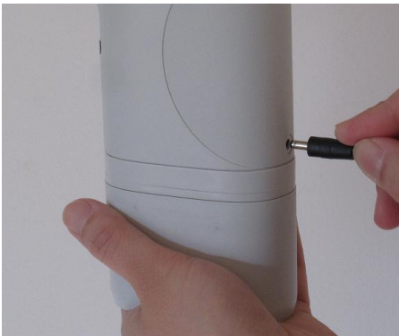
Figure 17. Charging Battery using the Power Supply
