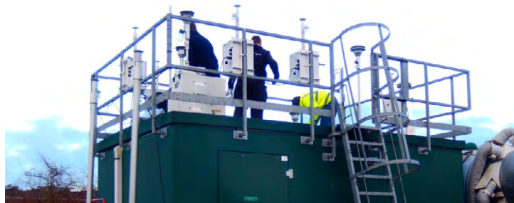
TSI's EDTPM2.5M, EDTPM10M and EDTDRXM were compared against European Reference Method Samplers, identified as PM10 and PM2.5 SEQ 47/50 manufactured by Sven Leckel GmbH.
