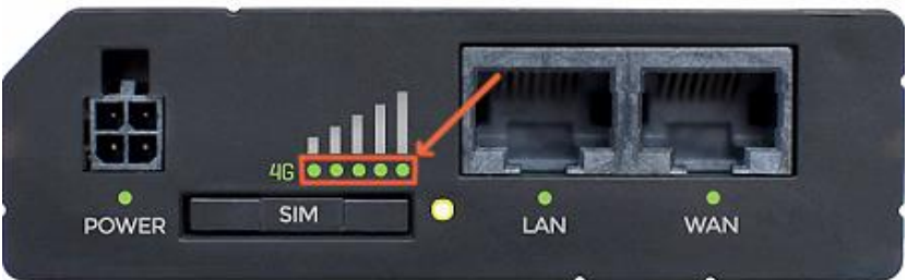
Figure 17: Signal strength LEDs
