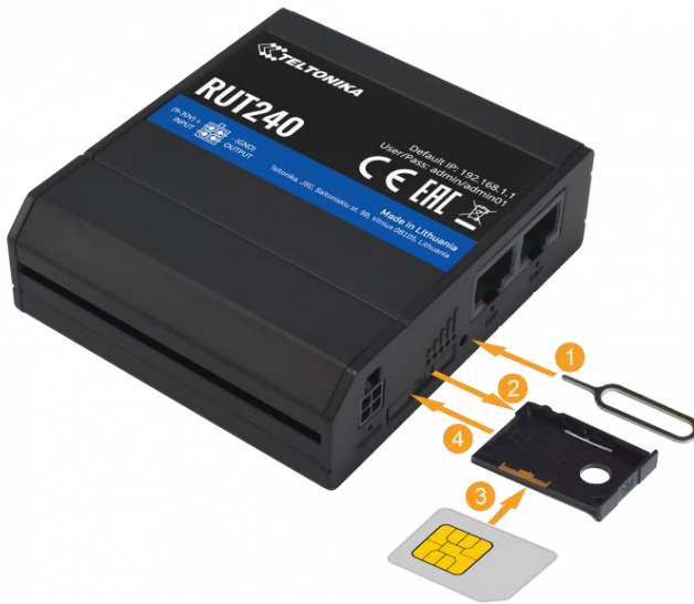
Figure 13: Installation of SIM card
