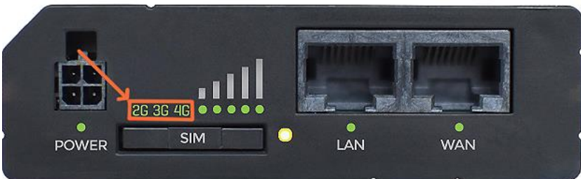
Figure 16: Connection status LEDs
