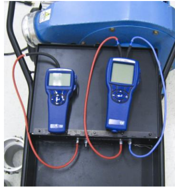
Figure 10. Connecting Instruments to PANDA Tester in High Flow Mode
