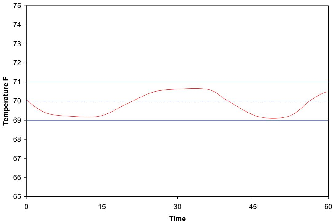
If TEMP DB is set to 1.0°F, and the TEMP SETP is set to 70.0°F, the controller will not take corrective action unless the space temperature is below 69.0°F or above 71.0°F.
