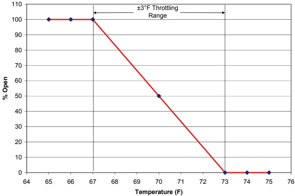
If TEMP TR is set to  $\pm 3.0^{\circ}\text{F}$ , and the TEMP SETP is set to  $70.0^{\circ}\text{F}$ , the reheat valve will be fully open when the space temperature is  $67^{\circ}\text{F}$ . Similarly, the reheat valve will be fully closed when the space temperature is  $73^{\circ}\text{F}$ .
