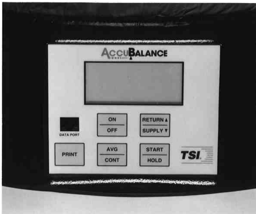
Figure 3. Electronic meter membrane switch
