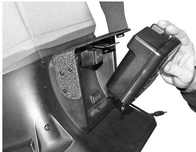
Figure 8: Attaching the Meter to the Capture Hood Base
